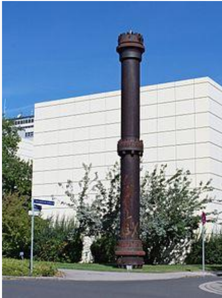
A historical (1921) high-pressure steel reactor for production of ammonia via the Haber process is displayed at the Karlsruhe Institute of Technology , Germany.
